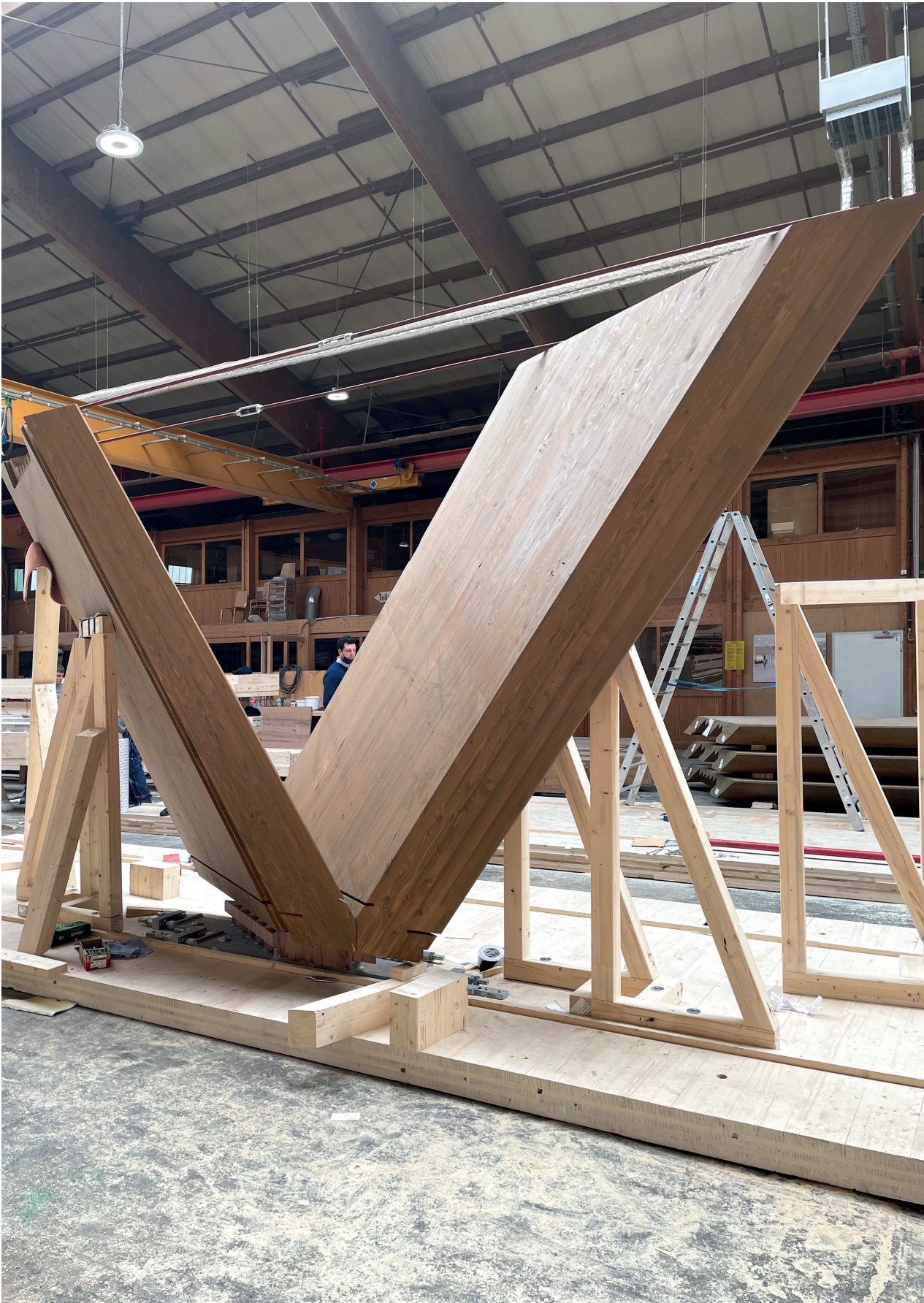
Prefabrication of the wooden supports in the factory
